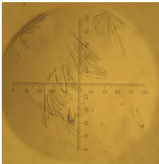
Figure 1 Crystals of the complex between rTxln-1 and trypsin grown from Hampton Crystal Screen 1 condition No. 27. These crystals are 0.3 \times 0.03 \times 0.01 \text{ mm} in size. A larger crystal (see Table 1) was used for data collection.
